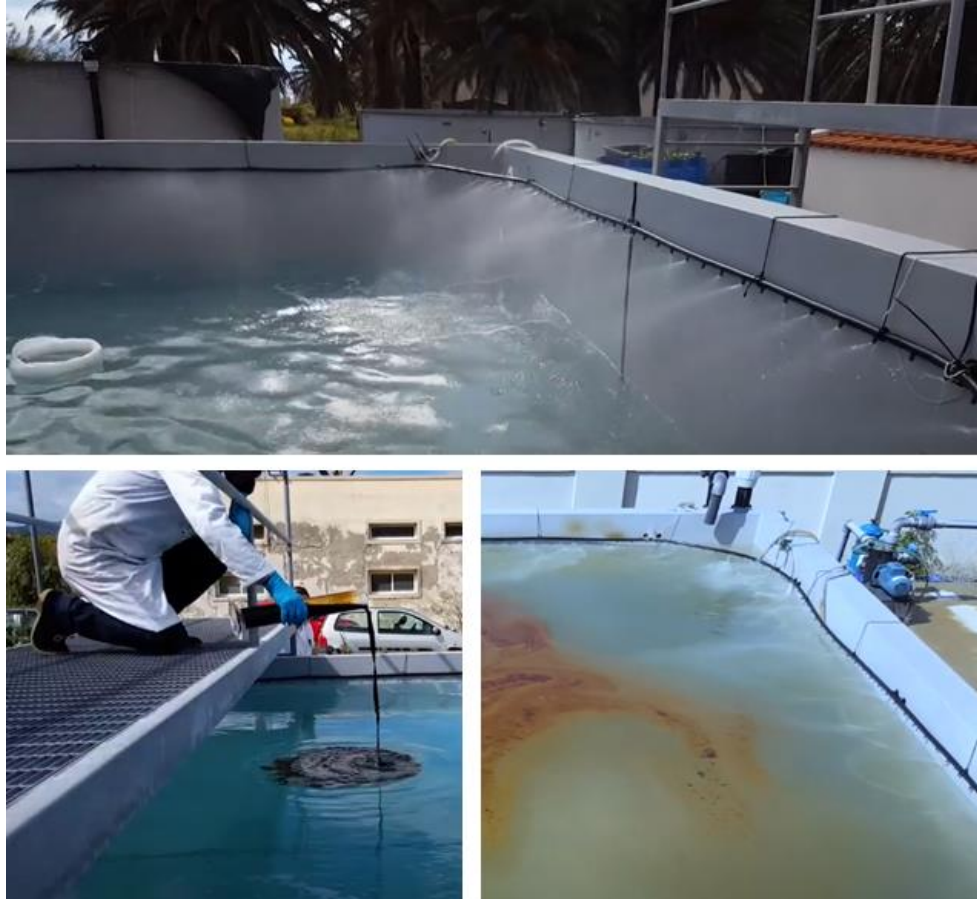
Figure 2 – Outdoor mesocosm facility at IRBIM-CNR of Messina. Different moment of activity related to simulation of oil spill in marine environment.
